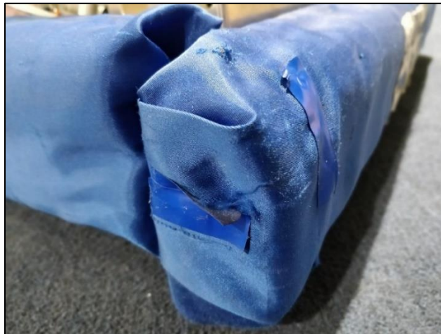
Figure 27: Bumper with tape covering ripped areas
