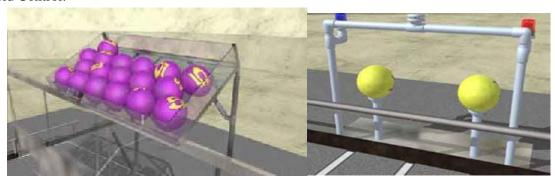
The Ball Release stores eighteen (18) Small Balls and is mounted above each Alliance Station.
