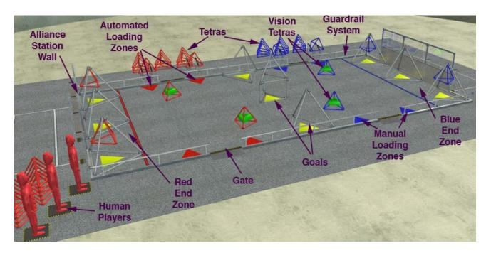
Note: The illustrations in this section of the manual are for a general visual understanding of the field and game only. Teams should refer to the drawings for exact dimensions and field construction. Note: Not shown here are the Human Player Loading Boxes (triangles) that are 48" on a side and are on the outside of the field directly opposite the Manual Loading Zones.
