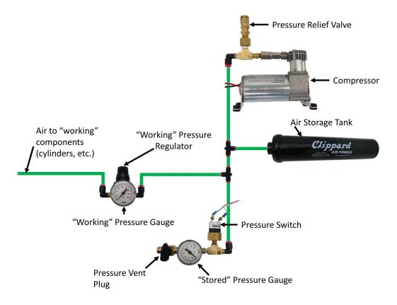
Figure 4-15: Pneumatic System Setup
