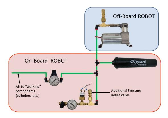
Figure 4-16: Off-Board Compressor with On-Board Regulator and Gauge
