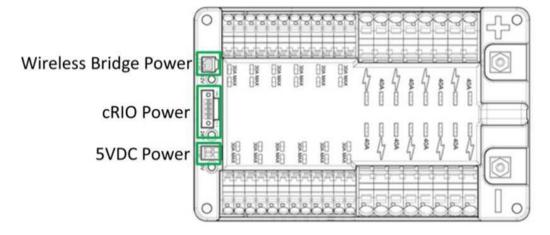
Figure 4-12: Wireless Bridge, cRIO, and 5VDC Power Connections
