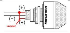
Figure 4-13: Jumper on RSL
