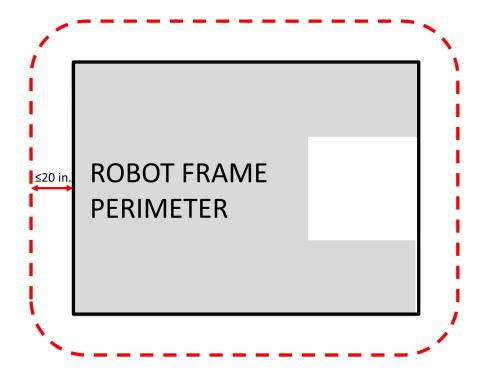
Figure 3-6: FRAME PERIMETER Extension
