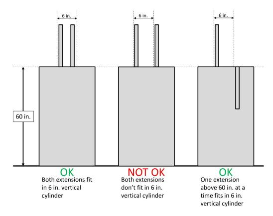
Figure 4-4: Multiple Vertical Extension Examples
