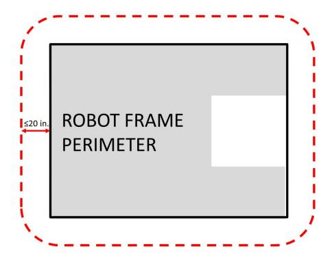
Figure 4-2: FRAME PERIMETER Extension
