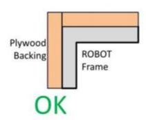
Figure 4-7: Hard Parts of BUMPER Corners
