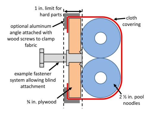
Figure 4-8: BUMPER Vertical Cross Section
