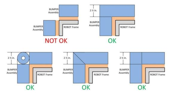
Figure 4-9: Soft Parts of BUMPER Corners
