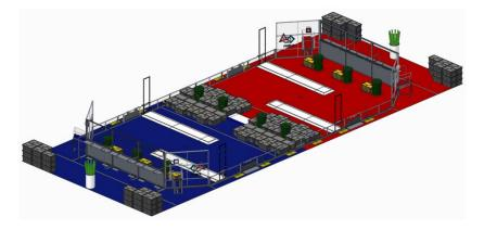
RECYCLE RUSH<sup>SM</sup> is a recycling-themed game played by two Alliances of three robots each. Robots score points by stacking totes on scoring platforms, capping those stacks with recycling containers, and properly disposing of pool noodles, representing litter. In keeping with the recycling theme of the game, all game pieces used are reusable or recyclable by teams in their home locations or by *FIRST*® at the end of the season.
