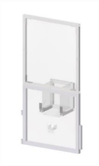
Four CLOUDS are positioned in each corner of the field, consisting of a 38" wide by 78" tall panel. DATALINKS are delivered through a 4" diameter hole 12" from the floor. GIGABYTES are delivered through a 10" diameter hole positioned 22  $\frac{3}{4}$ " from the floor. CLOUDS can hold up to 7 GIGABYTES before having to release them.
