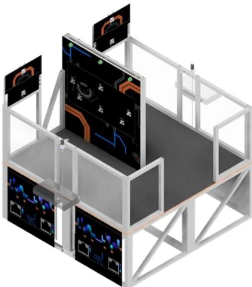
The NETWORK HUB is an 8-foot square 3-foot-high platform at the center of the field. There is an elevator on each side that is used to receive DATALINKS from the robots and bring them to the human players inside the structure. DATALINKS can then be hung on hooks to activate individual NODES. The NETWORK HUB starts with one DATALINK for each alliance that cannot be used until teleop.
