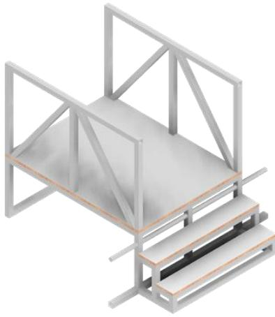
The BRIDGE's height is 22 inches. Robots on the alliance with the lower score may travel under the bridge to move between their CLOUD and NODES faster. LEDs will indicate which alliance has access at the time.
