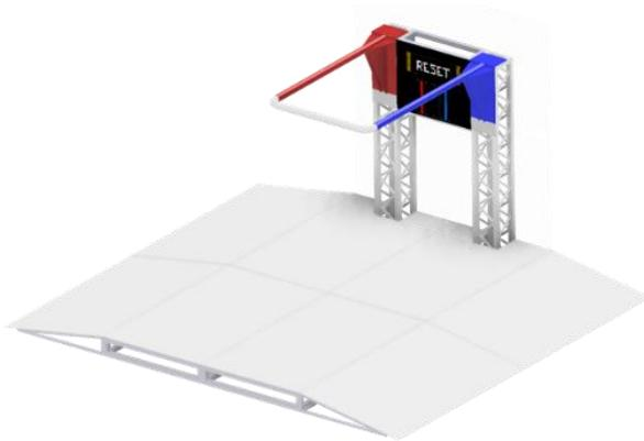
The RESET RELAY is a 3-inch diameter bar attached to the NETWORK HUB which is 8 ½ feet above the ground. It can hold 2 robots on the colored sides and 1 on the neutral side.
