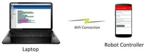
A developer uses a laptop, Chromebook or even a tablet to connect to the Blocks Programming mode server that resides on the *FTC Robot Controller*. The developer uses a Javascript-enabled browser to create and edit the programs, and then saves the programs directly onto the Robot Controller.
