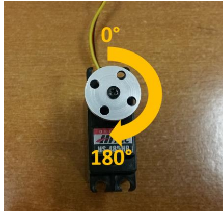
Figure 108 - A typical servo motor can rotate to and hold a position from 0 to 180 degrees.
