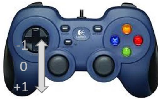
Figure 67 - The Y value of the joysticks range from -1 in the topmost position to +1 in the bottommost position.
