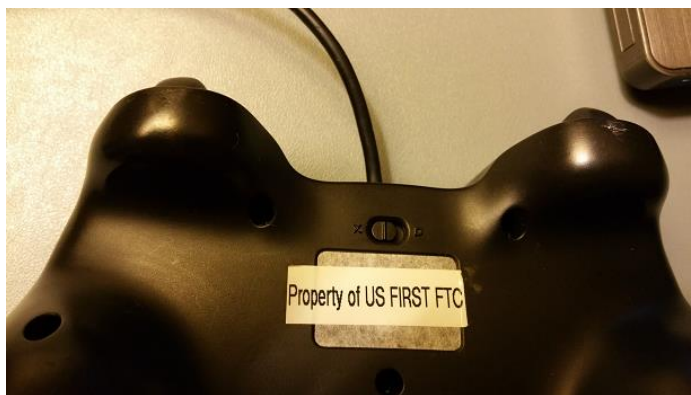
Figure 83 - Make sure the switch is in the "X" position.
