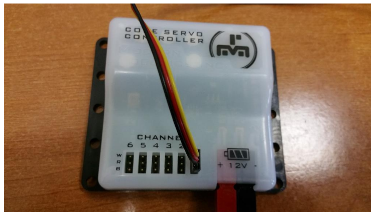
Figure 97 - Make sure to line up the yellow, red and black wires of the servo with the matching letter (“
