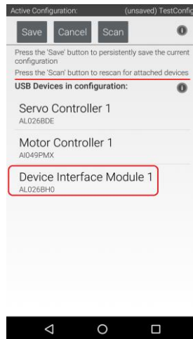
Figure 134 – Touch the Device Interface Module listing to edit its list of connected devices.
