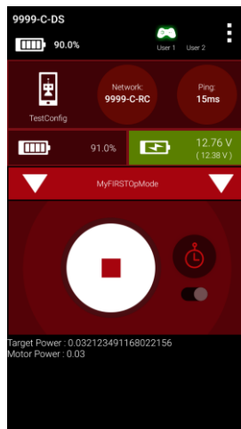
Figure 94 - The left joystick should control the motor. Telemetry data should appear in lower left hand corner of screen.
