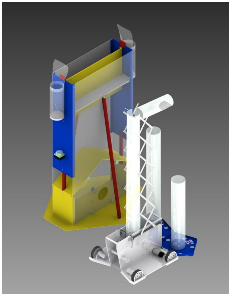
Figure 49 CAD/Lead Screw, Brackets, Lifts, and Ball Guide
