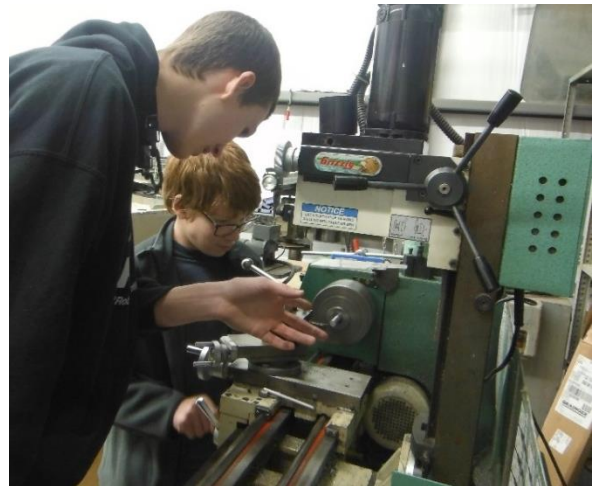
Turn Down Lead Screw
