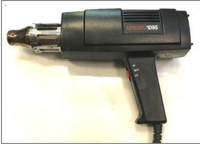
Figure 9: Heat Gun for Shrink wrap insulation.
