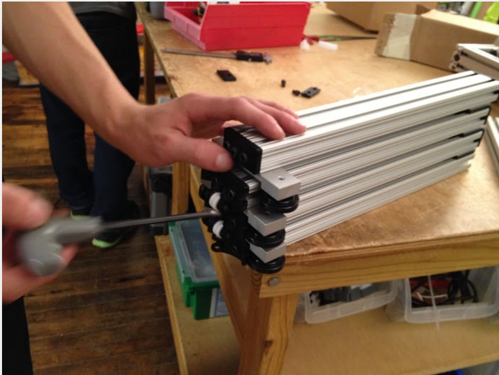
Slide lift with custom 3D printed pulley brackets
