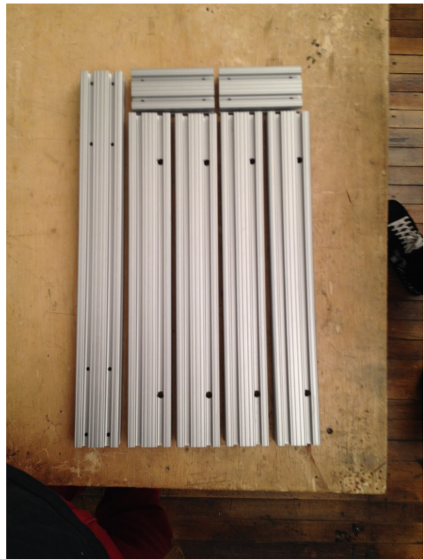
80/20 chassis rails ready for assembly
