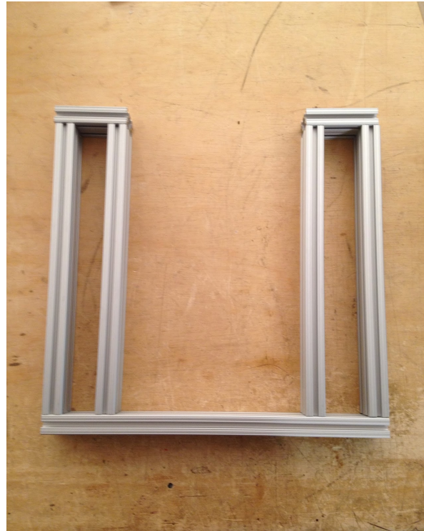
Cut 80/20 chassis rails ready for drilling
