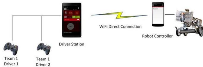
One Android phone is mounted on the Robot and is called the Robot Controller. The other phone sits with the team drivers and is called the Driver Station. The Android devices run special apps (the *FTC Robot Controller* app and the *FTC Driver Station* app respectively).
